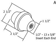
All insulators made from UL recognized flame resistant fiberglass reinforced polyester compound.
